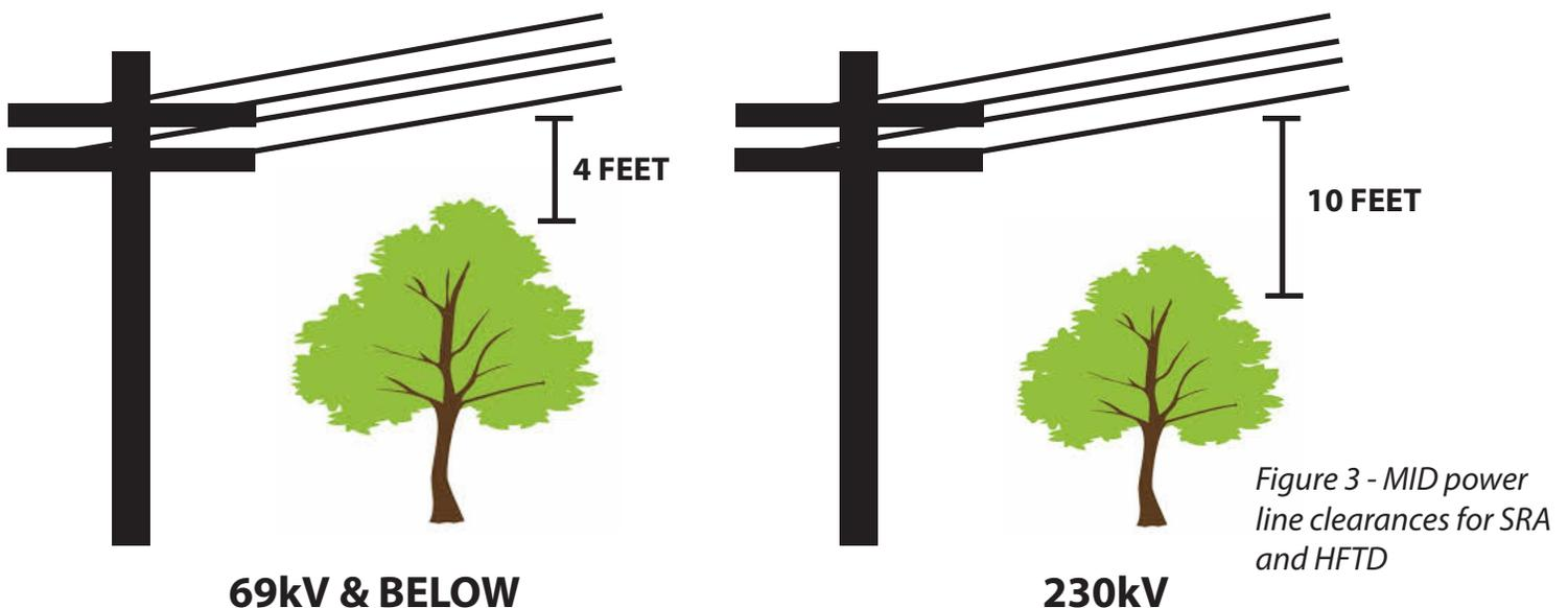
*Figure 3 - MID power line clearances for SRA and HFTD*
