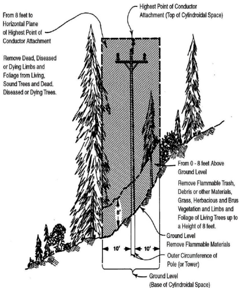
**TO COMPLY WITH PRC-4292, MID MAINTAINS 10 FEET RADIAL CLEARANCES AROUND POLES AND STRUCTURES WHERE NON CAL FIRE APPROVED EQUIPMENT ARE USED IN SRA'S AND TIER-2 AREAS.**
