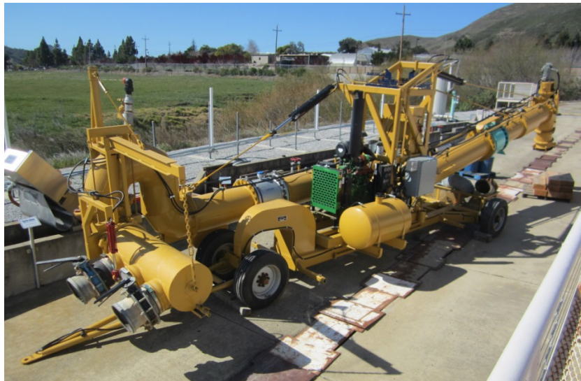
Figure 3. Pumping system for IID jack gate characterization
