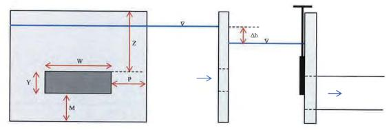
Figure 4. Flow through a submerged orifice plate
