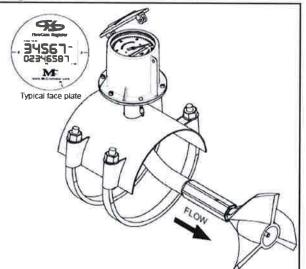
McCrometer will also mount a reverse-facing propeller on a standard open flow meter, which can be mounted on stands above low pressure pipelines.
