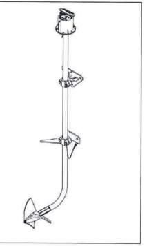
A commercially available package that includes a reverse propeller meter and trash-shedding fixed vane, plus flow straighteners, is available from RSA.
