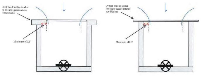
Figure 5. Installation of orifice
